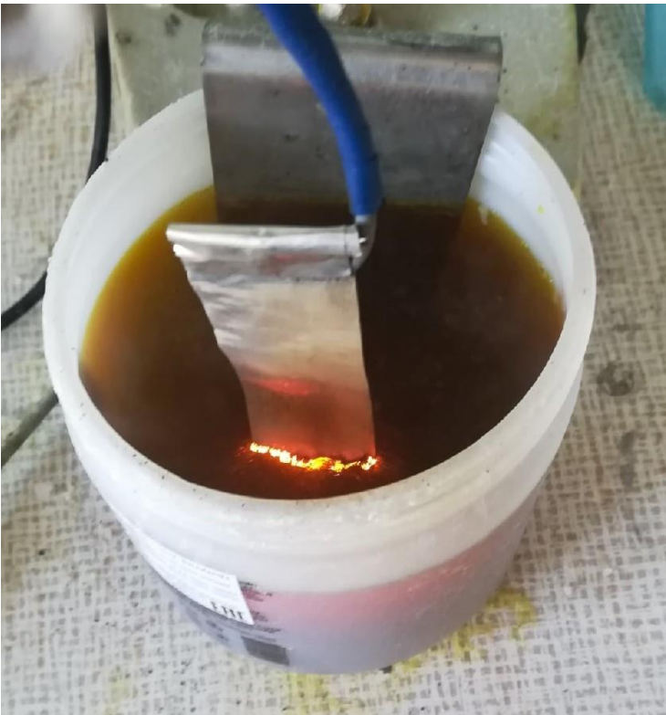
Fig. 3. The process of electrolyte-plasma polishing in 4%FeCl 3 +2% C 2 H 2 O 4 .
