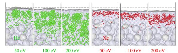
During the first 100 fs the incident He ion manages to move a large distance across the target and create a few small regions of local overheating, but after 500 fs the ion loses almost completely its energy in collisions with atoms. So high penetrating ability of He ions due to their small size leads to the infiltration of implanted atoms into deeper layers of the material, causing slow collapse of pores that continues even after the formation of an solid layer.
