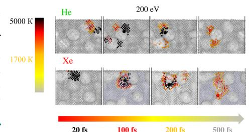
The impact of the Xe ion of the same initial energy leads to the formation of a much more extended overheated region, which exists longer. So the pore collapse happens most rapidly. However, at certain fluence this process stops due to the formation of a sufficiently extended continuous layer, which prevents incident ions from reaching underlying pores.
