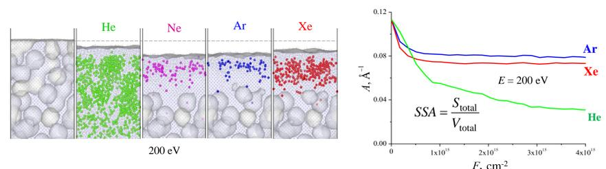
The depth of the solid layer at the steady state also depends strongly on the sort of ions and their energy. This value is almost linearly proportional to the ion energy at low energies.
