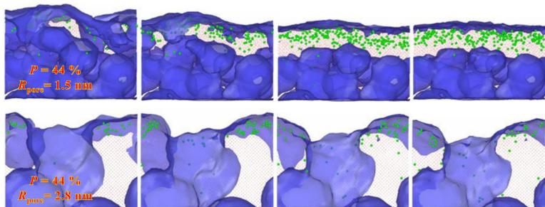
Molecular dynamics simulation of Ar ion irradiation showed that ion impacts initiate near-surface solid layer formation that prevents the material from penetration of active plasma species. The appearance of this layer is the most probable for the film with low porosity and pore radius.
