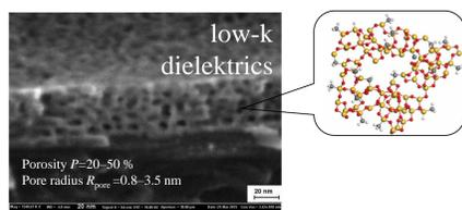
Active plasma species can easily penetrate into deeper layers of these films, damage material structure. This results in decrease of dielectric constant.
