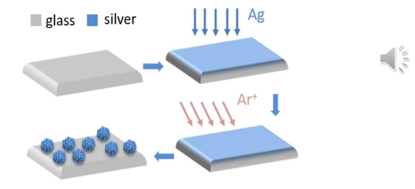
Schematic process of the fabrication of the samples
