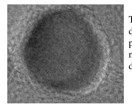
TEM studies of the nanoparticles revealed high degree of their monocrystallinity. However, no preferred NPs orientation is observed: various nanoparticles situated on the substrate surface have different orientation.
