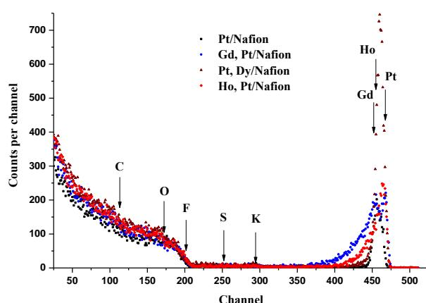
Fig. 5. RBS spectra of  $^4\text{He}$  ions from surface of Nafion membrane with layers formed by IBAD of platinum and rare earth metals
