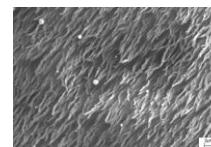
Fig. 2. SEM image of the Nafion™ N115 membrane with layer formed by the IBAD of platinum [2]
