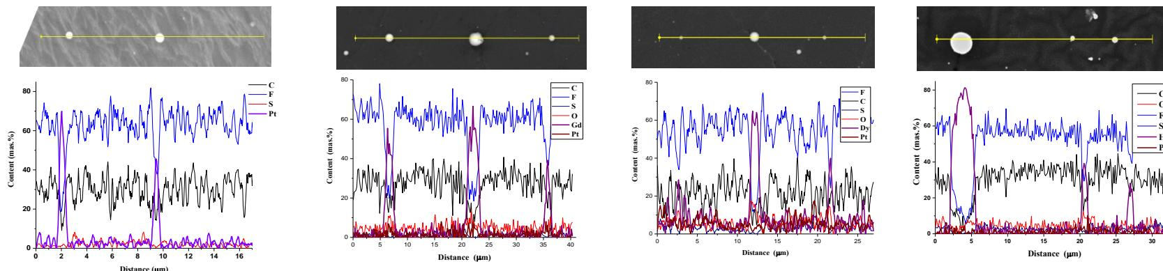
Fig. 3. SEM images and distributions of atoms of elements across the scanning line (according EDX) over the surface of the Nafion™ N115 membrane with investigated layers
