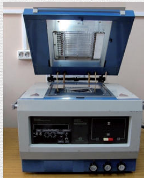
Special "Impuls-6" equipment for ILP annealing
