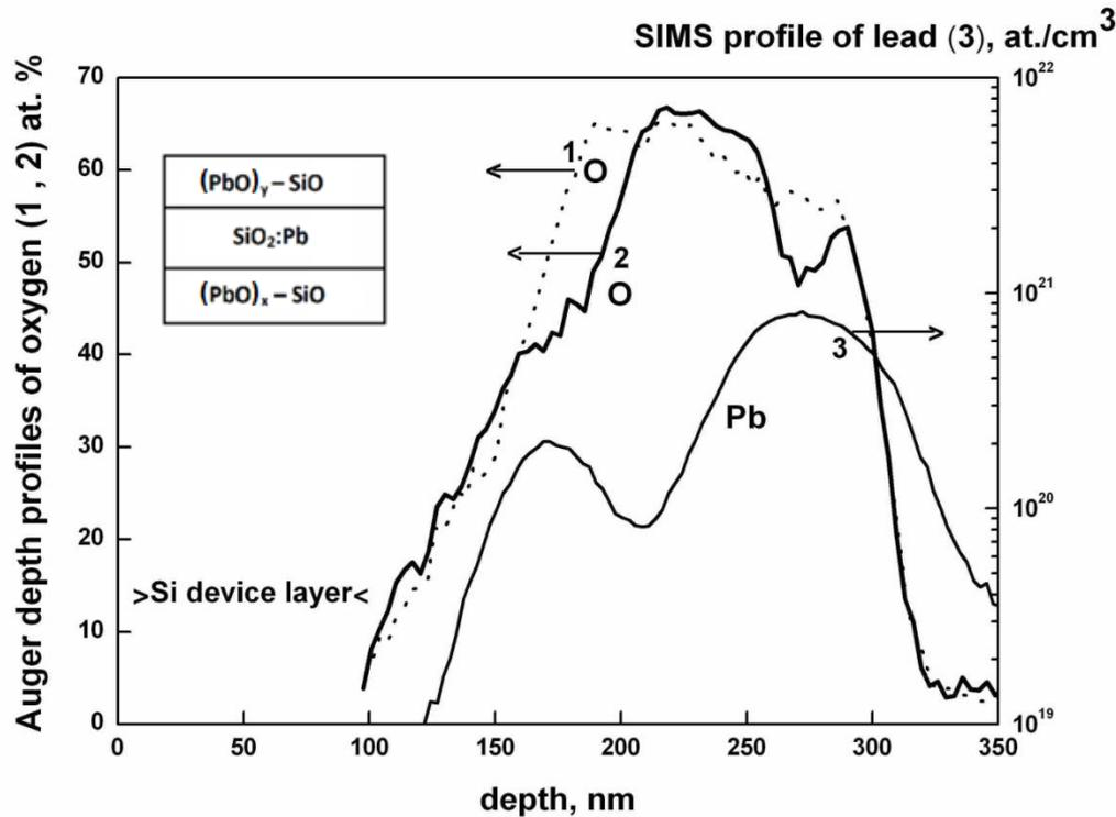
SIMS profile of lead (curve 3) and profiles of AES oxygen analysis (left: curve 1 and 2) for implanted samples after annealing at 1150°C for 8 hours. Curve 1 corresponds to the reference sample (without lead ion implantation).
