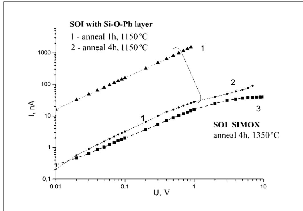
The figure shows the current-voltage characteristics of experimental samples (1, 2) in comparison with the standard SIMOX structure (3) with a BOX layer thickness of 0.37  $\mu\text{m}$ . As shown the electrical breakdown characteristics of SOI structures with a lead-silicate insulator are close to those of standard SIMOX structures. In this case, the annealing temperature is 200°C lower for the same annealing duration.
