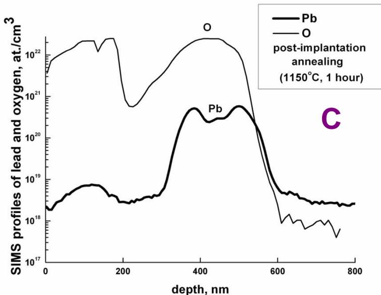
The figures show SIMS profiles of the distribution of main implanted components. The lead is non-uniformly distributed over depth, and its highest concentration observed at the boundaries with silicon. This is due to a segregation of the lead into inhomogeneous regions between adjacent phases. As a result, a three-layer insulator structure is formed. In its central part, the oxygen content reaches the stoichiometric level of SiO<sub>2</sub> - 67 at.%.
