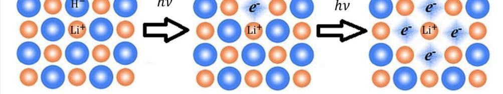
The accumulation of defects around one Li atom leads to the formation of metallic lithium with a crystal lattice
